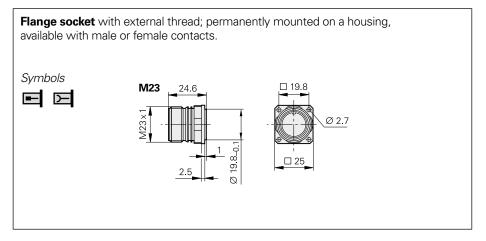
The pins on connectors are **numbered** in the direction opposite to those on couplings or flange sockets, regardless of whether the connecting elements have
