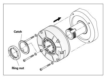
Shaft coupling with ring nut and catch
