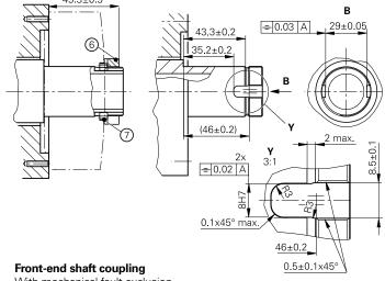
With mechanical fault exclusion (for further dimensions, see "Without mechanical fault exclusion")
