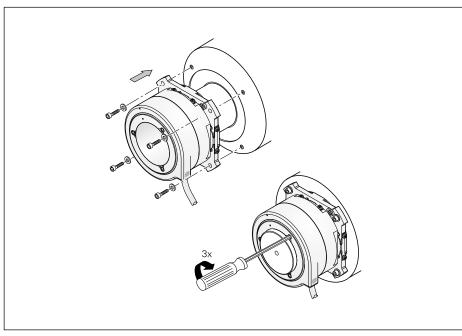
Mounting an ECN 200 with  $\varnothing$  50 mm hollow shaft
