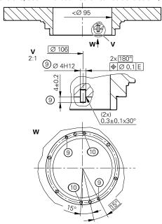
= Shown rotated by 45° = Accessory: Ring nut ID 336669-16 = Accessory: Catch ID 817921-04 = Screw penetration > 10 mm
