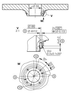
= Screw penetration > 10 mm = Accessory: Ring nut ID 336669-11 = Accessory: Catch ID 817921-03 = 2x spring pins ISO 8752 - 4x10 - St
